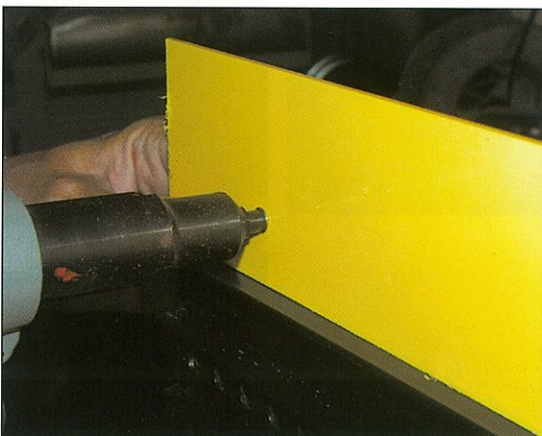
◀ Connections are easily formed by riveting and welding.
